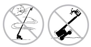
Use extreme care and slow speeds while driving the machine in the stowed position across uneven terrain, debris, unstable or slippery surfaces and near holes and drop-offs.
